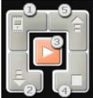
and has five different buttons. While we are talking about the controller I will give a brief description of each button's function. Button #1 - Opens the NXT window which allows you to rename the brick and delete programs or files. Button #2 - Downloads programs to the NXT brick. You will use this button more than any other to
