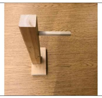
Insert the 5" Round Dowel into the Furring Strip all the way thru. Glue if possible.
